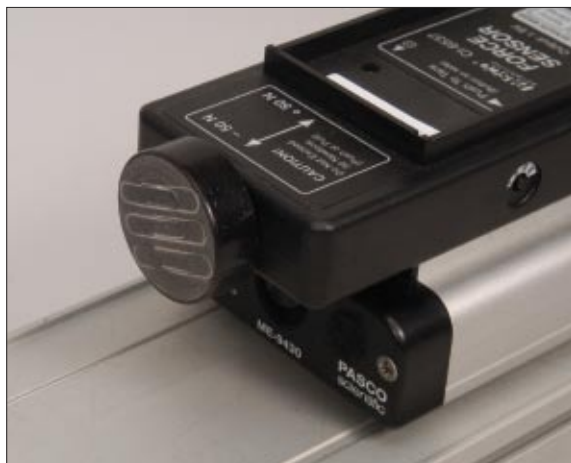
Fig. 2. Three paper clips are imbedded in a nylon disk. The front of the disk is slightly sanded so that the three paper clips clearly show. The nylon disk can be attached to a force sensor to digitally record the force exerted on the paper clips.
