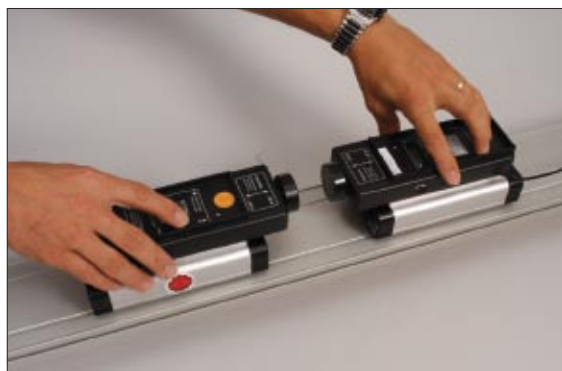
Fig. 3. Three paper clips, imbedded in a nylon cylinder, as shown in Fig. 2 are mounted on one force probe. A second force probe holds a nylon cylinder of the same dimension that contains a small neodymium magnet. For convenience sake we have mounted the force sensors on dynamics carts.
